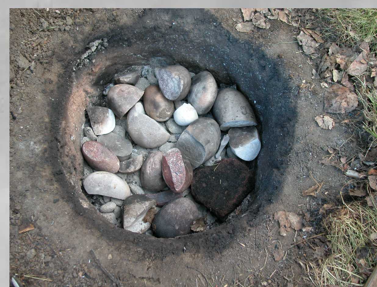
Fire pit during experiment, major fracturing occurring with discoloration.
